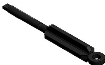
The PE401N travel restrictor restricts the amount of opening on the lower sash to a typical set distance of 100mm dependant on the customers requirements. This is adjusted by the position in which the restrictor is fitted on the stile of the sash. The travel restrictor is fixed in place using two fixings which are screwed through either side of the sash. This gives the restrictor a secure fixing and hides the screw fixings from sight.
